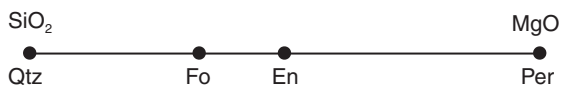
FIGURE 13 SiO 2 -MgO chemographic diagram assuming only Qtz, Fo, En, and Per are stable.
