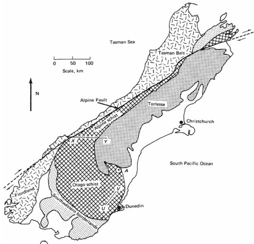
FIGURE 10 Geologic sketch map of the South Island of New Zealand, showing the Mesozoic metamorphic rocks east of the older Tasman Belt and the Alpine Fault. The Torlese Group is metamorphosed predominantly in the prehnite-pumpellyite zone, and the Otago Schist in higher grade zones. X-Y is the Haast River Section of Figure 11. From Turner (1981).
