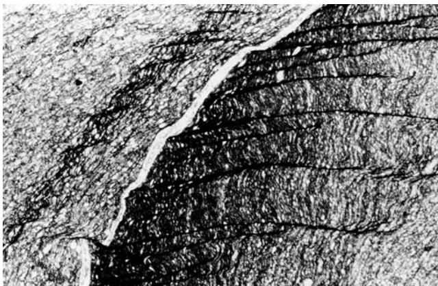
FIGURE 32 Pelitic schist with three s-surfaces. S_0 is the compositional layering (bedding) evident as the quartz-rich (left) half and mica-rich (right) half. S_1 (subvertical) is a continuous slaty cleavage. S_2 (subhorizontal) is a later crenulation cleavage. Field width \sim 4 mm. From Passchier and Trouw (2005). Copyright © with permission from Springer-Verlag.
